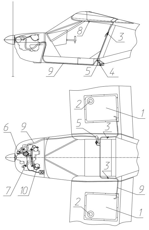
Fig. 2. Fuel system schematic
