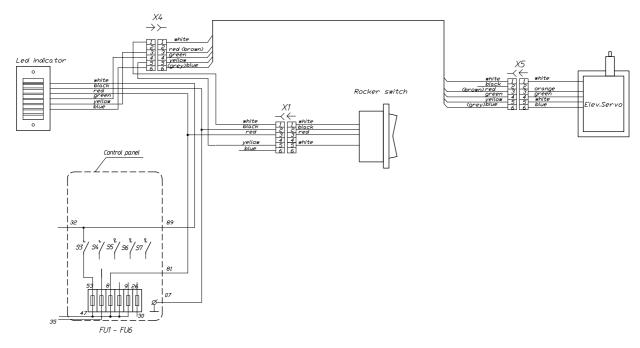
Fig. 18. Wiring diagram for installation of the electric servo of elevator trim tab
