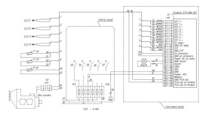
Fig. 16. Wiring diagram for installation of FLYdat
