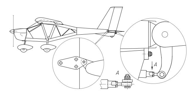
fig. 25. Disconnection of the horizontal tail
