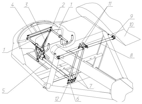
Fig. 6. Control system of flaperons (drooping ailerons)
