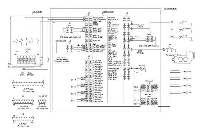
Fig. 20. Wiring diagram for installation of DYNON FlightDEK D-180
