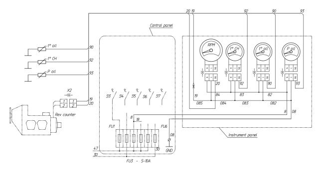
Fig. 15. Wiring diagram for installation of analog engine instruments
