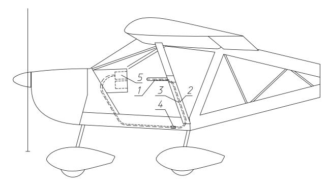
Fig. 12. Full and static pressure system
