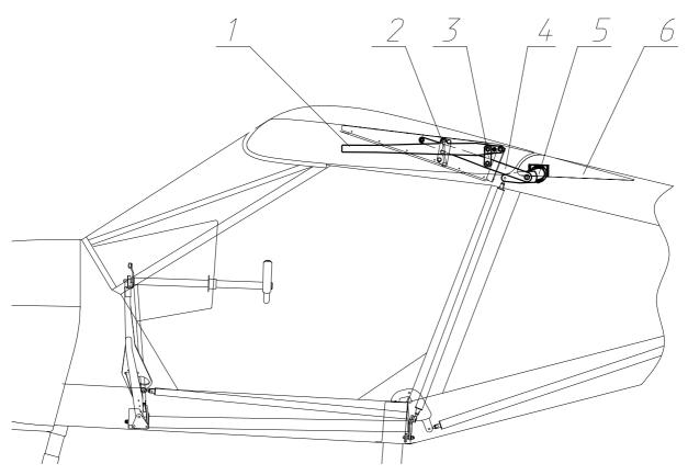
Fig. 7. Flap extension mechanism
