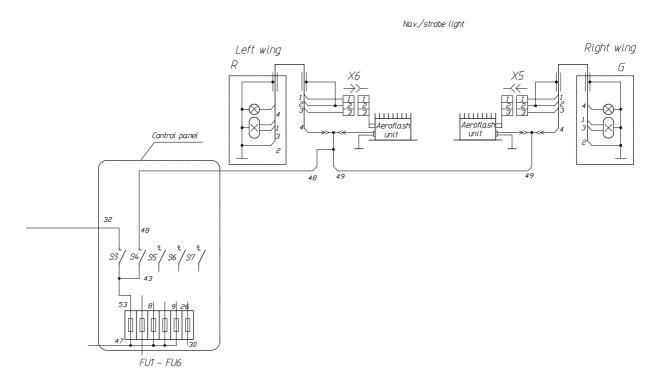
Fig. 14. Wiring diagram for installation of strobes
