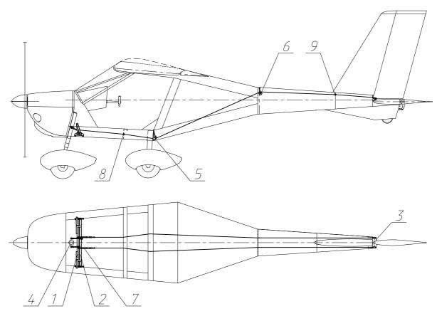
Fig. 5. Rudder and nose landing gear control system
