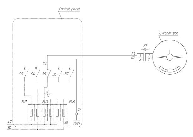
Fig. 19. Wiring diagram for installation of gyro horizon
