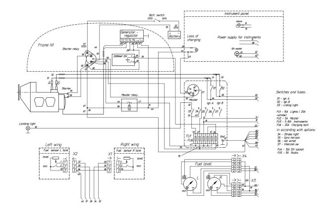
Fig. 13. Wiring diagram of A-22LS electric system (main)
