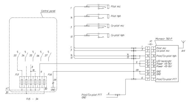
Fig. 17. Wiring diagram for installation of Microair 760-P radio
